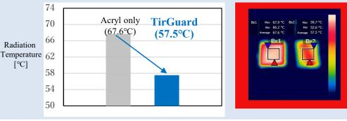
Acrylic resin coating with TirGuard added and an acrylic resin coating were placed on a 70°C hot plate. The radiation temperature was measured using a far-infrared camera from a distance of 50 cm above.
