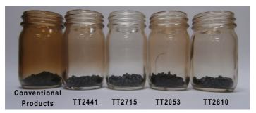
Masterbatches are put in glass bottles and allowed to stand for 1 hour in a 300° electric furnace.
